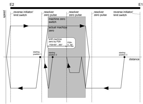
The speed used for find machine zero is specified by P3; the accelerating and braking time by P7.
